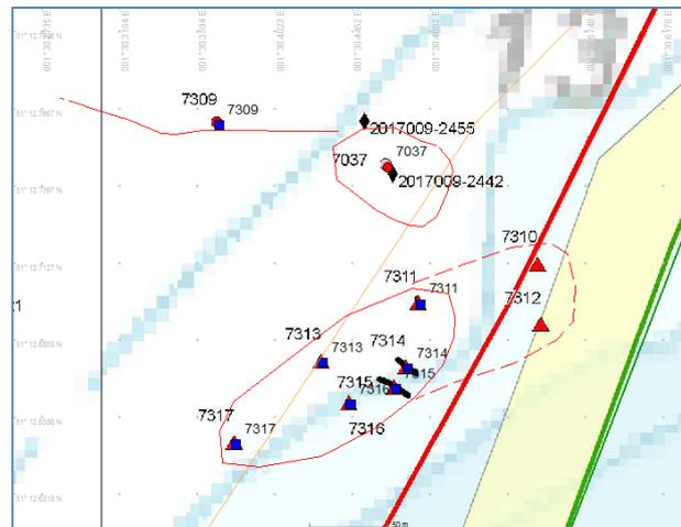
This is one of the most interesting targets in the survey area. The area of the targets is clearly very different to the rest of the survey area and the targets are in a group which is comparatively small in size, which suggests that this is the remains of a shipwreck or a military aircraft crash site. The targets are also not magnetic so are unique in this dataset and very rare anywhere else. Together this group of targets are clearly man made and of archaeological interest.
